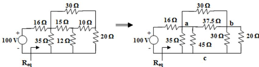
$$R_{ab} = \frac{15 \times 10 + 10 \times 12 + 12 \times 15}{12} = \frac{450}{12} = 37.5 \Omega$$
