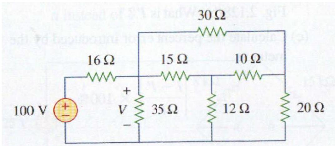
We need to find  $R_{eq}$  and apply voltage division. We first transform the Y network to  $\Delta$ .
